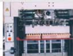
Non-stop feeder with pre-loading device, also taking pallet right off the press
